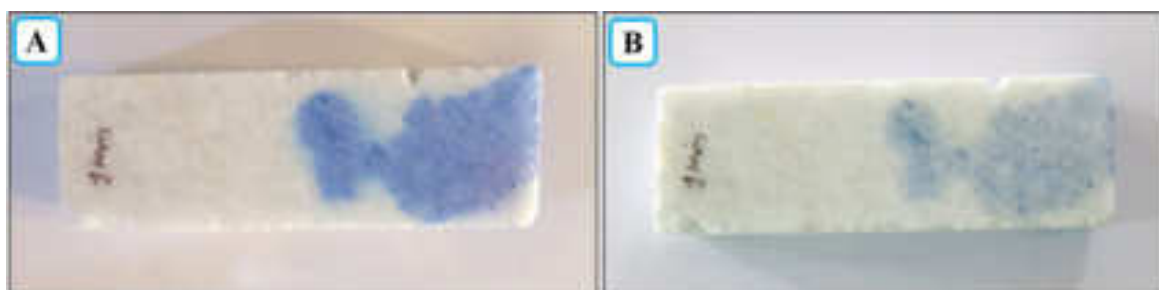
Fig. 6: Photograph of self-cleaning photodegradation test by MB, (A) before UV exposure and (B) after 30 hrs exposure to UV irradiation.
