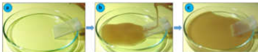
Figure 6. a-c) Self-cleaning behavior of superhydrophobic coating.
