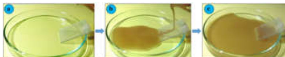
Figure 6. a-c) Self-cleaning behavior of superhydrophobic coating.
