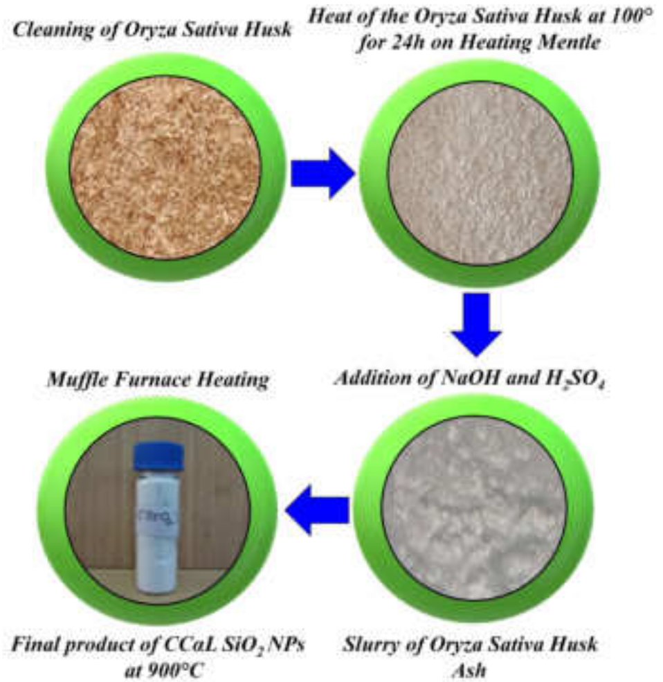
Fig. 1 a Flow diagram for the synthesis of crystalline cristobalite alpha low silicon dioxide nanoparticles (CC \alpha L SiO 2 NPs) from Oryza sativa husk and b Schematic representation of CC \alpha L SiO 2 NPs anode half-coin cell
